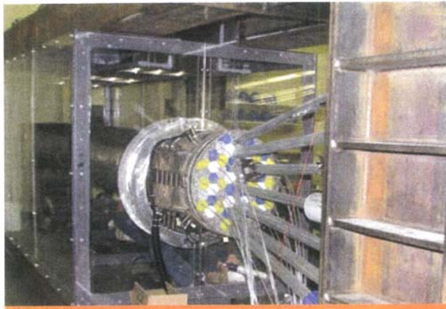
Laboratory testing new technology to monitor the bridge cable corrosion underwater
